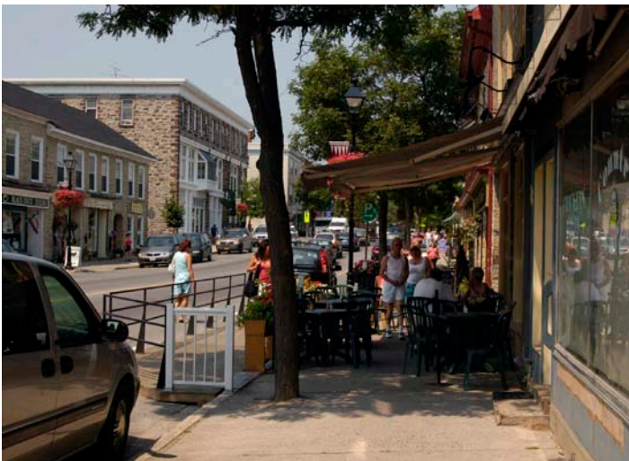
Provision for on-street parking reduces the number of driveways and minimizes the pedestrian-vehicle conflict in Perth, Ontario
