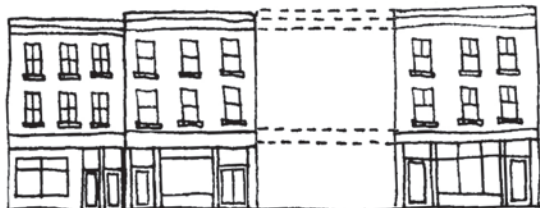
Consistent horizontal alignment of façade elements
